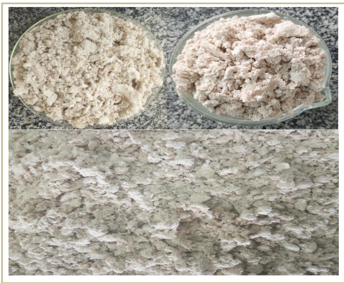
Figure 4.1. Bleached and freeze-dried cellulose
